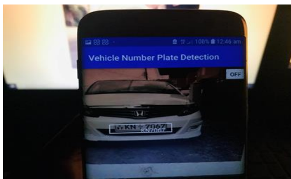
Figure 4: Number plate detection camera screen with flash light & zoom feature
