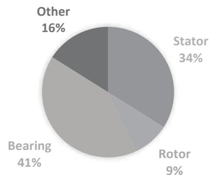
Fig. 1 Common faults in an induction motor
