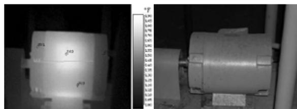
Fig. 3 - A motor which is been heated [7]
