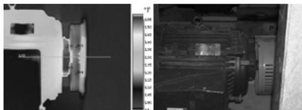
Fig. 2 - An induction motor with faulty bearing [7]
